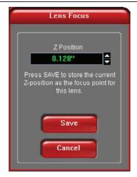
**4.** Click on the Calibrate button within the Lens Size box of the System Tab. The following window appears. Click on Save to accept the new Z Position. Your 20 Lens has now been calibrated.
