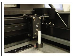
2 Using the UP and DOWN arrow buttons, either on the machine (enter the Z Menu) or in the UCP, bring the Z-axis table up. Using the appropriate Focus Tool for the lens installed (the standard is 2Q other Focus Lens Kits are optional), focus directly on the surface of the table.
