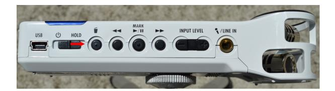
To disable the buttons, slide the power switch upward to HOLD. To enable use of the buttons again, slide the power switch back to the middle position.
