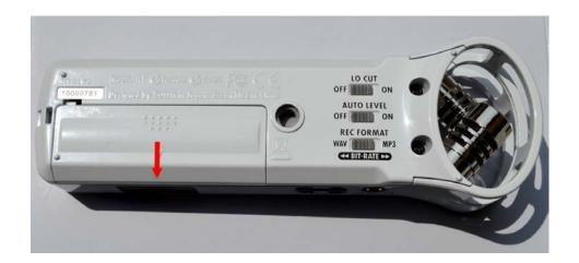
Open the case while pressing here and then insert the battery respecting the +/- orientation.
